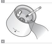
Empty the water in the tank, add a small amount of warm water ( do not exceed  $40^{\circ}\text{C}$  ) (  $103.9^{\circ}\text{F}$  ) , and a few drops of neutral cleanser. Use the cleaning brush provided to clean the internal surface of the water tank. Gently rinse all the soap out of the water tank after washing, do not use dishwashing liquid.
