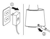
Remove the AC adapter from the electrical outlet and then remove the plug from the main unit.
