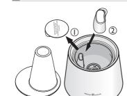
Remove the glass cover first, and then remove the retaining plate from the vent hole and replace it with the provided waterproof cap.
