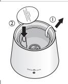
Remove the water level label and place the retaining plate into the vent in the tank. ( as shown in diagram left ) .
